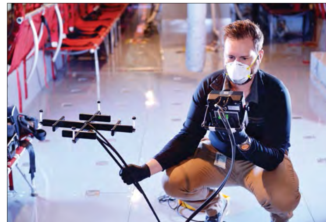
Brett Edwards, Universal Energy Systems research scientist, tests fog particles dispersed throughout a KC-135 Stratotanker aircraft April 8 at the 155th Air Refueling Wing, Nebraska National Guard Air Base, Nebraska. Air Mobility Command, in coordination with the National Strategic Research Institute at the University of Nebraska and Defense Advanced Research Projects Agency, examined airflow and particles to assess ways to eliminate virus transmission to aircrew when transporting Covid-19 patients.
